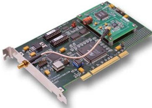
**Figure 2.** GPS Creations PCI GPS hardware.
