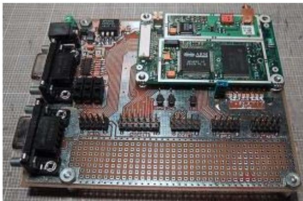
**Figure 3.** Signav MG5001 receiver on support board.
