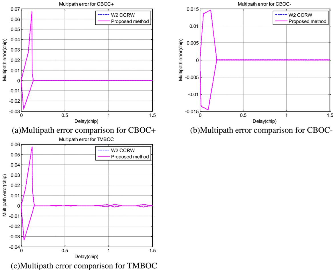
**Figure 6.** Multipath error comparison between W2 CCRW and proposed method in CBOC and TMBOC ( $GW_{W2}=1/3$  chip,  $GW_{BRW}=1$  chip, infinite bandwidth).
