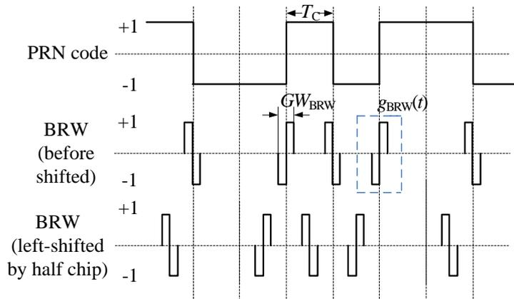
**Figure 3.** Example of locally generated PRN code and corresponding BRW.
