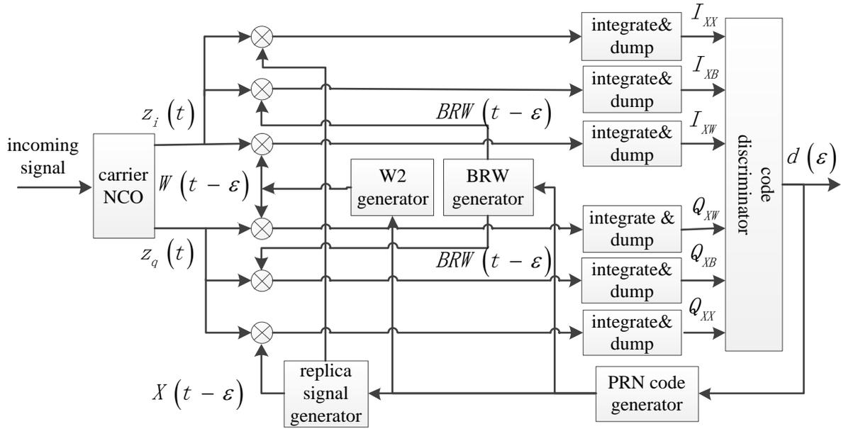
**Figure 4.** Block diagram of receiver code loop of proposed scheme.
