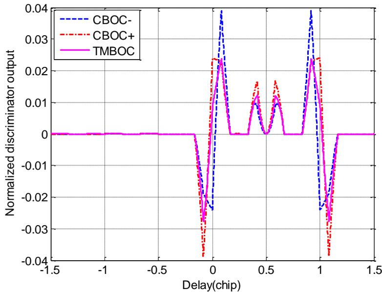
**Figure 5.** Normalized discriminator output of proposed method in CBOC and TMBOC ( $GW_{W2}=1/3$  chip,  $GW_{BRW}=1$  chip, infinite bandwidth).
