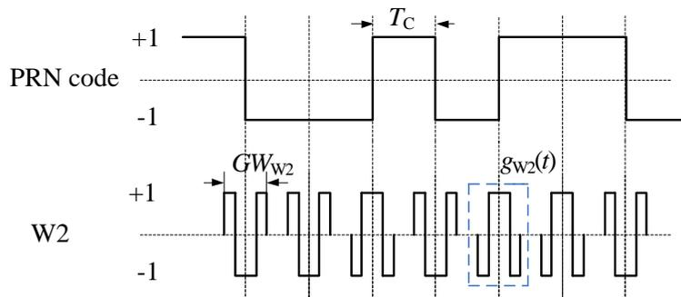
**Figure 1.** Example of locally generated PRN code and corresponding W2 waveforms.
