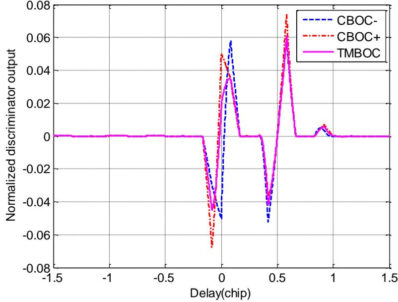
**Figure 2.** Normalized discriminator output of W2 in CBOC and TMBOC ( $GW_{W2}=1/3$  chip, infinite bandwidth).
