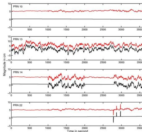
**Fig. 3** Comparison of converted single-difference residuals (*top curve in each subplot*) with simulated values (*bottom curve in each subplot*) for reference satellite (PRN 10) and three multipath-contaminated satellites (PRNs 13, 14 and 22)
