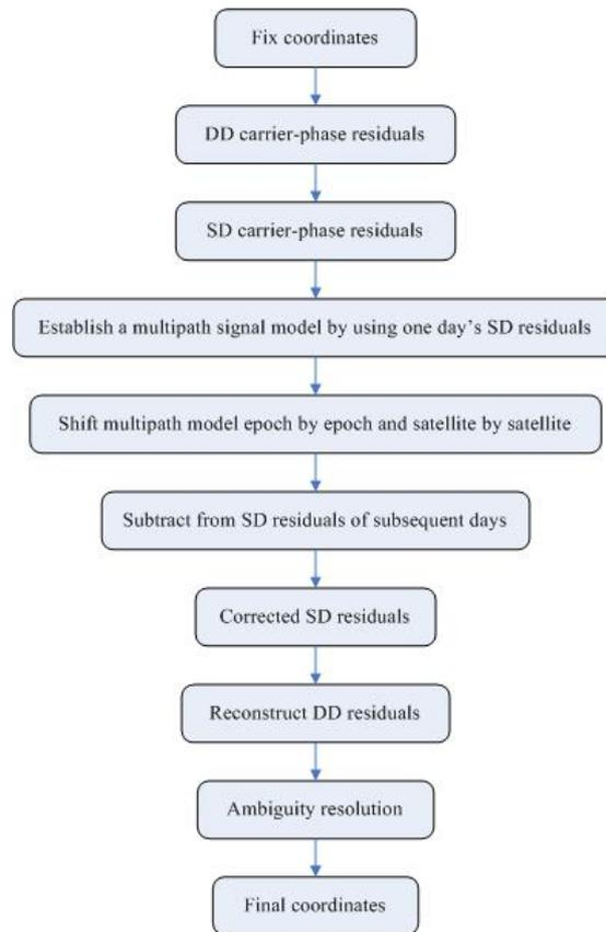
**Fig. 1** Sidereal filtering procedure based on GPS single differences (DD: double-difference; SD: single-difference)
