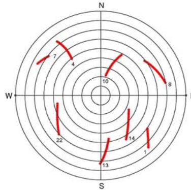
**Fig. 2** Sky plot of GPS satellites over the reference station
