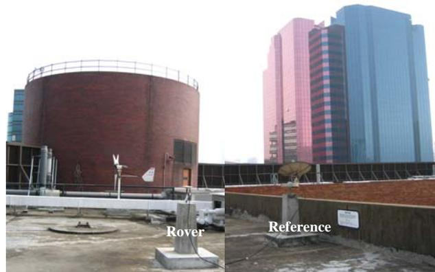
**Fig. 4** Reference and rover stations and site environment
