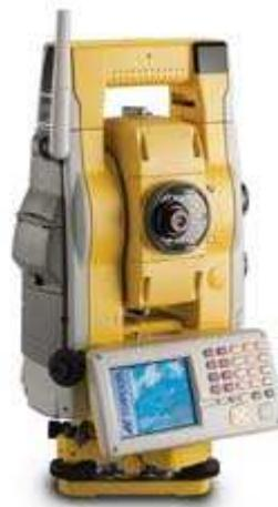
Fig. 2. Cable-Free Robotic Total Station
