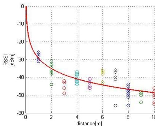
**Figure 1.** RSSI attenuation according to the elapsed distance
