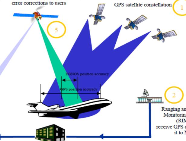
Mission Control Centres (MCC): process GPS data to determine errors
