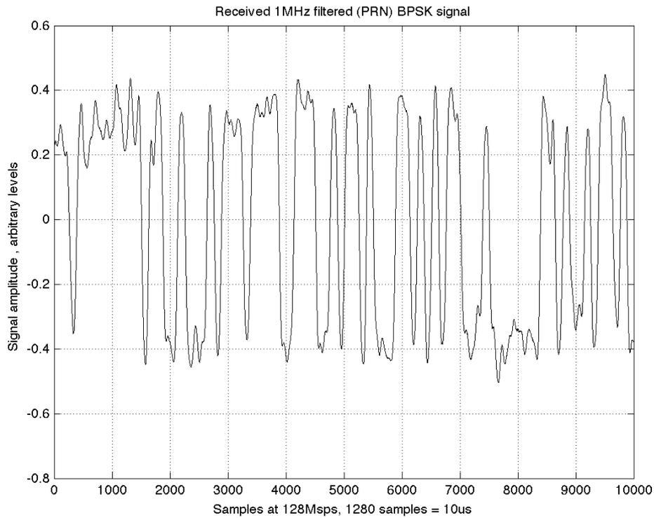
**Figure 2.** C/A spreading code appearing as BPSK
