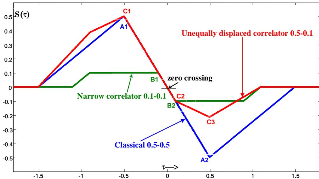
**Figure 3.** S-functions for different correlator displacement
