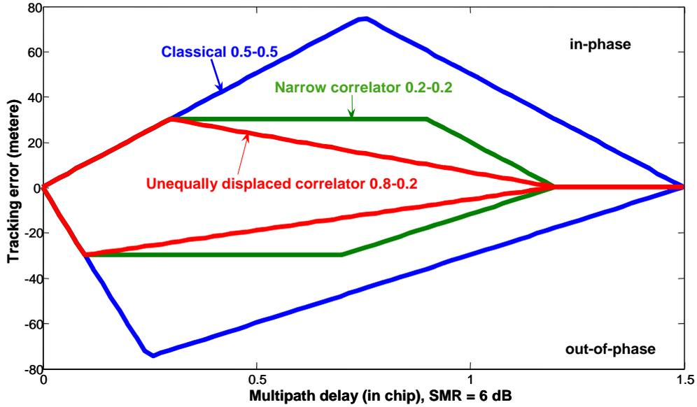
Figure 4. The multipath error analysis
