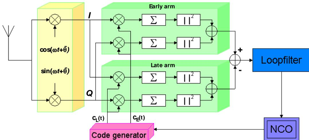
Figure 2. Tracking loop for the delay estimation (DLL)
