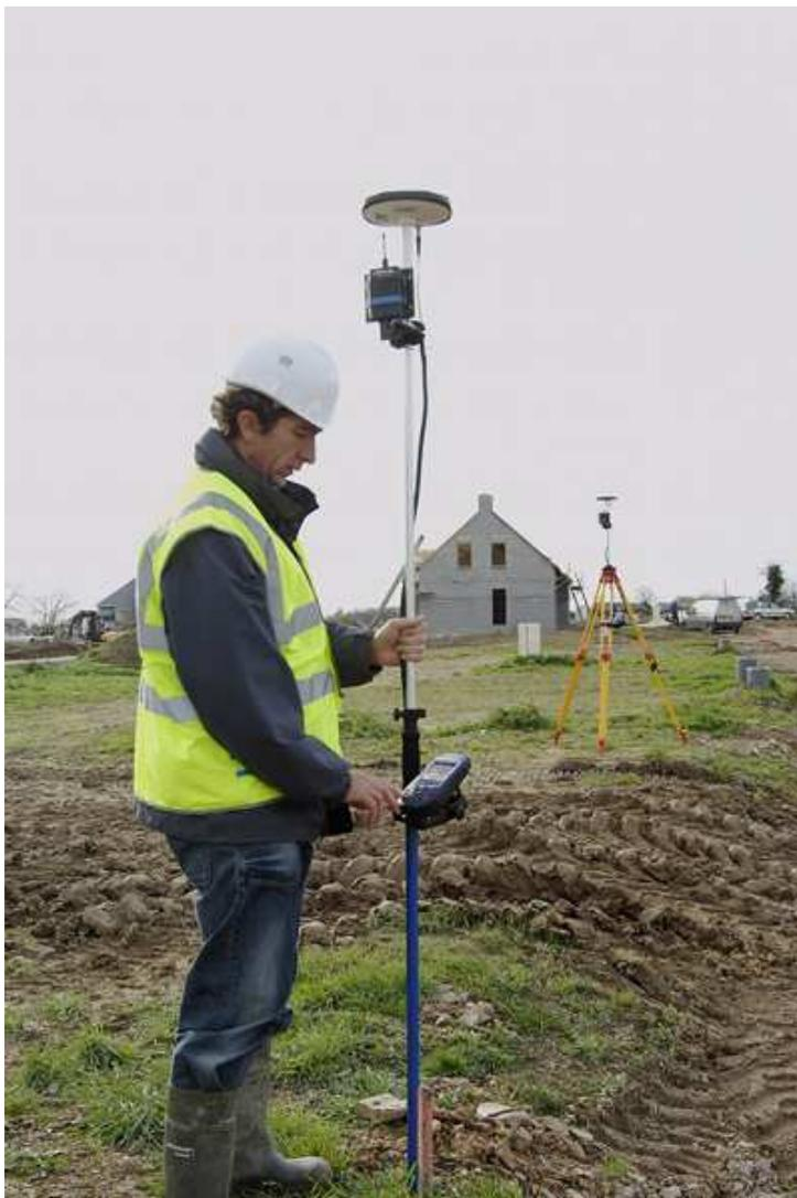
**Photograph 1.** ProMark3 RTK GPS Receiver - Rover & Base
