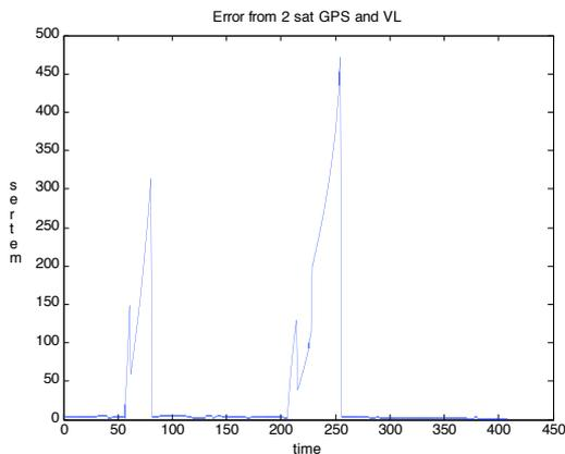
**Figure 8: Error when only two GPS satellites trackable**
