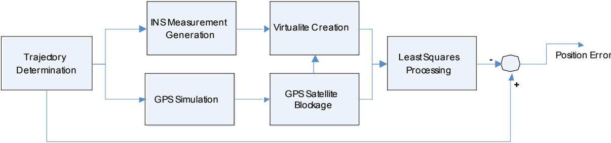
Figure 1: INS and GPS simulation diagram
