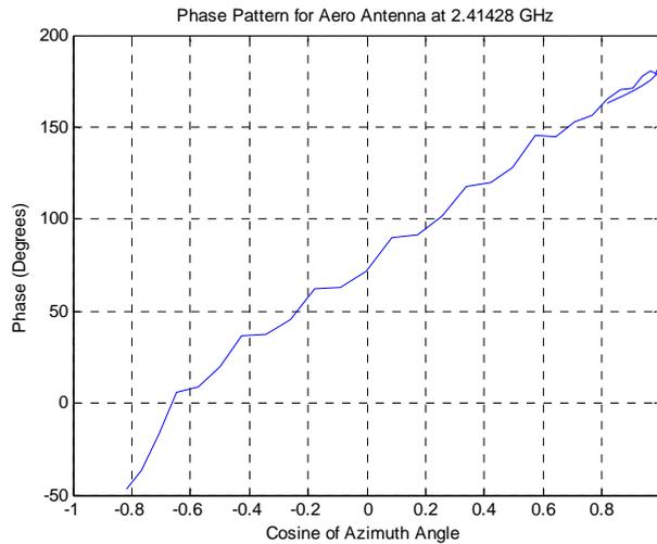
**Figure 3:** Phase pattern of Aero antenna at vertical polarization and frequency of 2.4143 GHz
