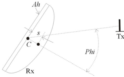
**Figure 2:** Experimental setup for Phase Centre determination
