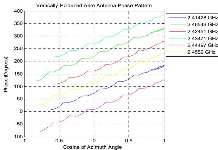
**Figure 4:** Phase patterns of AUT with vertical polarization
