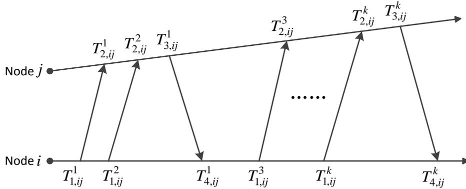
**Figure 1.** Two way timing message exchange between node  $i$  and node  $j$ .
