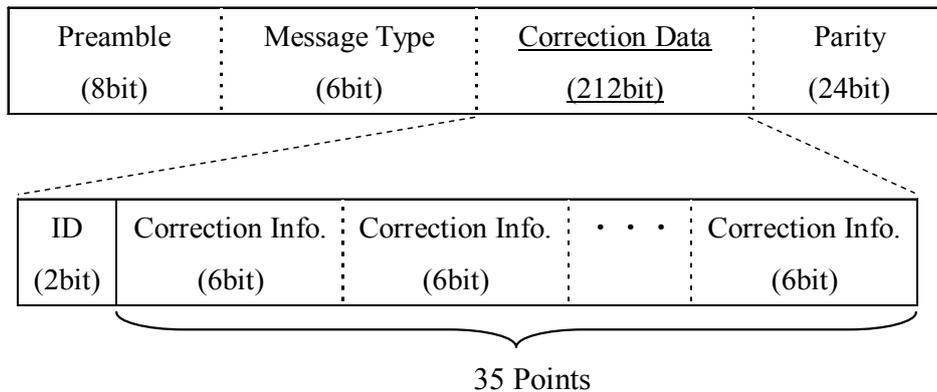
**Figure 5.** Design of Tropospheric Daly Correction Message
