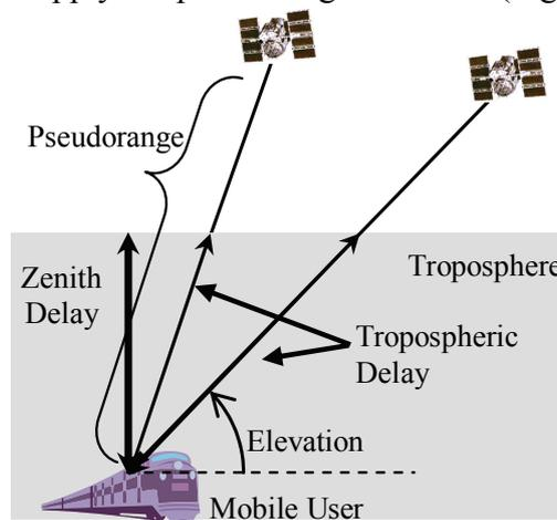
**Figure 2.** Tropospheric Delay Estimation from ZTD
