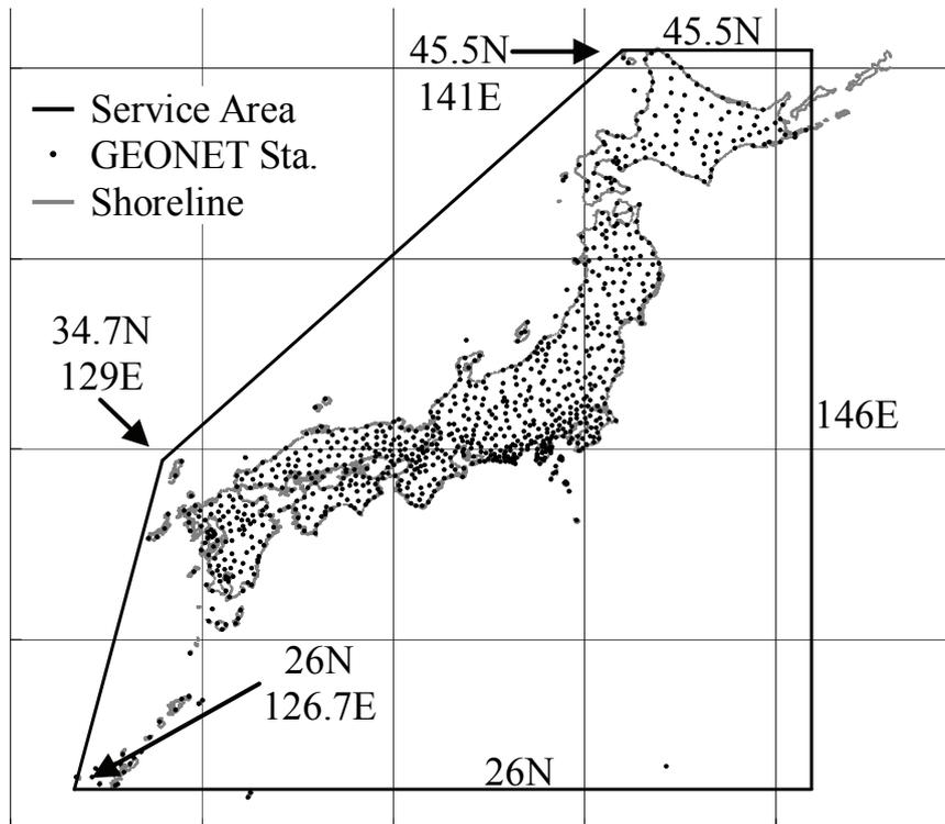
Figure 1. Service Area of L1-SAIF and GEONET Stations
