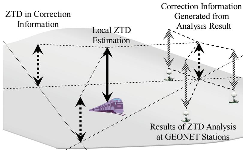
**Figure 4.** Generation of Correction Information and Estimation of Local ZTD
