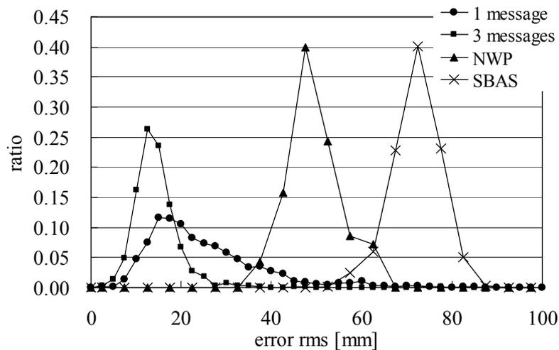
Figure 10. Distribution of Correction Accuracy
