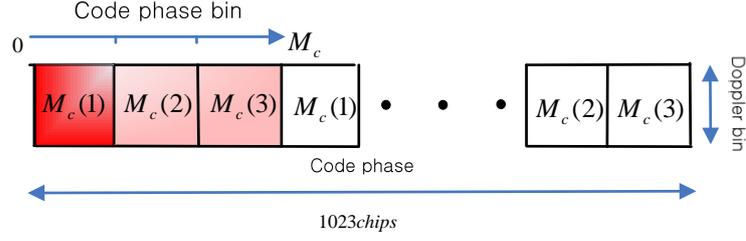
**Figure 4.** Code phase search using multiple correlators
