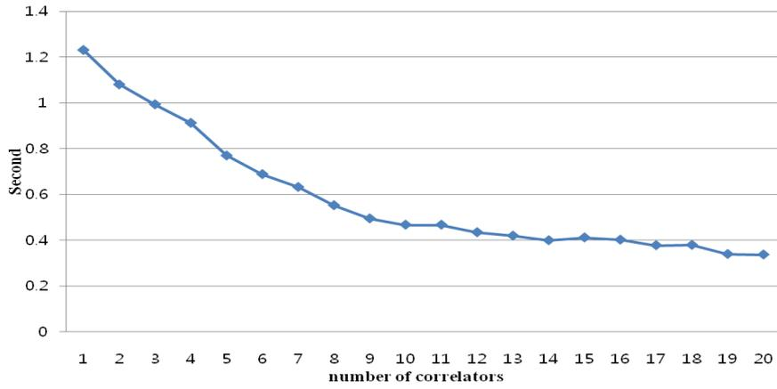
**Figure 11.** Average acquisition time of the proposed method
