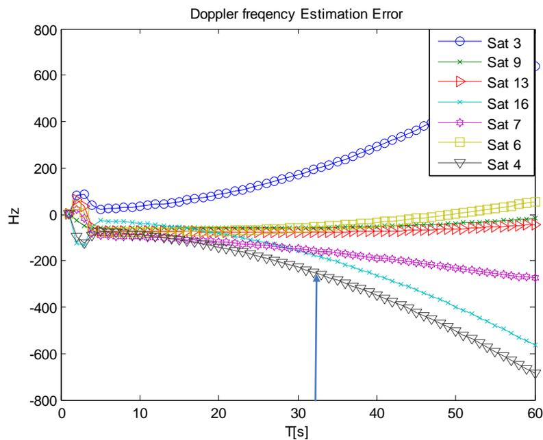
**Figure 10.** Doppler frequency estimation error
