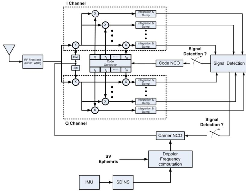
**Figure 5.** Acquisition structure of a GPS receiver
