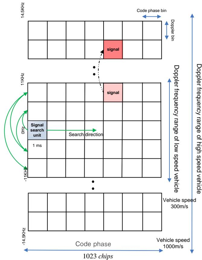
Figure 2. Signal search area in high speed vehicles
